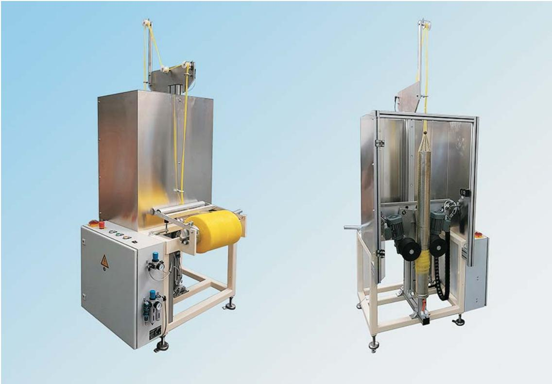
The automatic sleeving machine GKV 3300 is being used for the mechanical loading of extruded netting material coming from a roll, onto filling tubes having a max. diameter of 160mm and a max. length of 1000mm. The machine is designed to run standard net rolls having a width of 310mm, an outer Ø of max. 300mm and an inner core Ø of 75mm.
